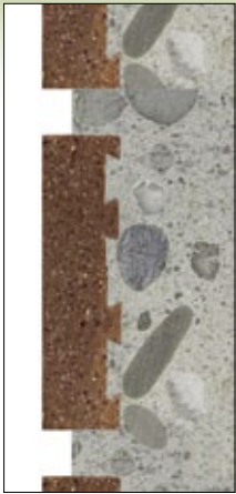
DOVETAILED BACK. Serves as a fastener for sure bond.
