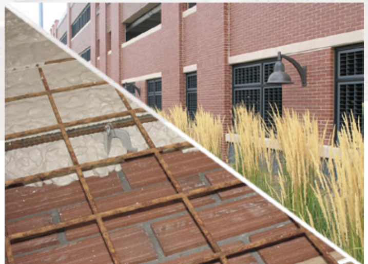
How the thin brick fits into the liner during panel production can directly affect the look of the finished project.
