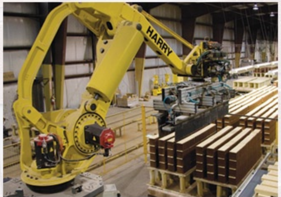
The above photo shows a robot- affectionately referred to as 'Harry' - unloading product and placing it on the inspection/packaging line in the METROBRICK manufacturing plant .
